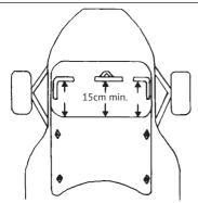
Lower end of bubbleshield showing minimum 15cm gap between shield and pedals. Also indicating the maximum 4 fixing points if shield attached to bodywork.
