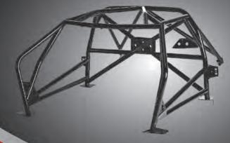
1.3.7. Removable Members. Should removable members be used in the construction of a ROPS, the demountable joints used must comply with an approved type (see drawings K21 to K30). The screws and bolts must be of adequate diameter and of ISO Standard 8.8 or better. FIA homologated demountable joints are also permitted.
